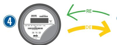
A bi-directional meter measures delivered electricity (DE) used from the grid (net consumer) and electricity returned (RE) to the grid (net producer). These values are both displayed on the meter for your convenience.
