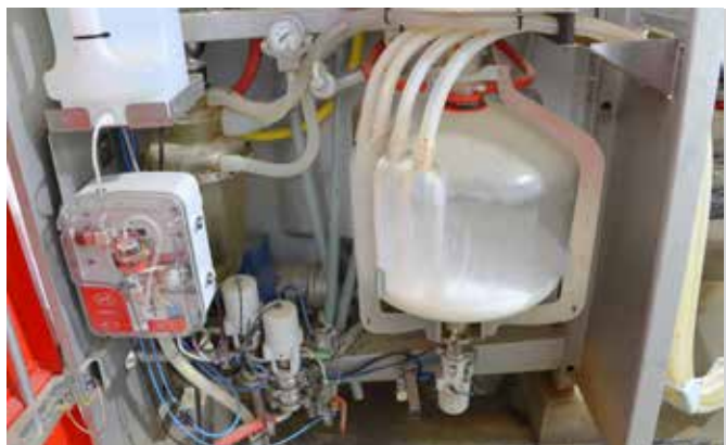
Pictured above: Astronaut A5 robotic milk receiver container and meter. Pictured right: Robotic arm control panel.
